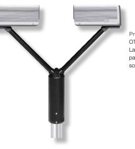
Precipitation measurement OTT Parsivel<sup>2</sup> – Laser-optical disdrometer for capturing particle size and velocity of liquid and solid precipitation
